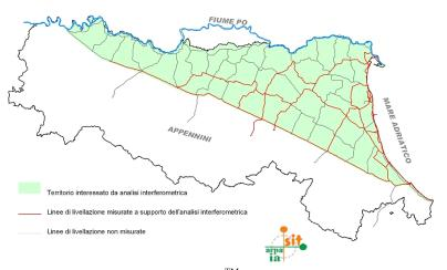
**Fig. 1** Area covered by PSInSAR<sup>TM</sup> interferometric analysis and levelling lines (in red the lines surveyed during the 2005 campaign).
